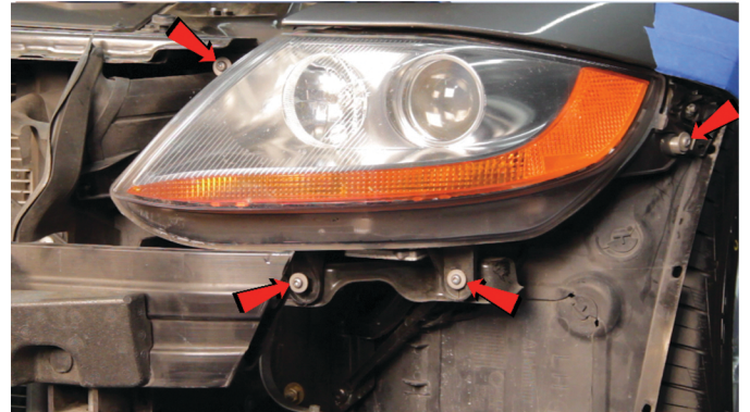
8) Remove [4x] T-25 Torx bolts securing the headlight to the body.
