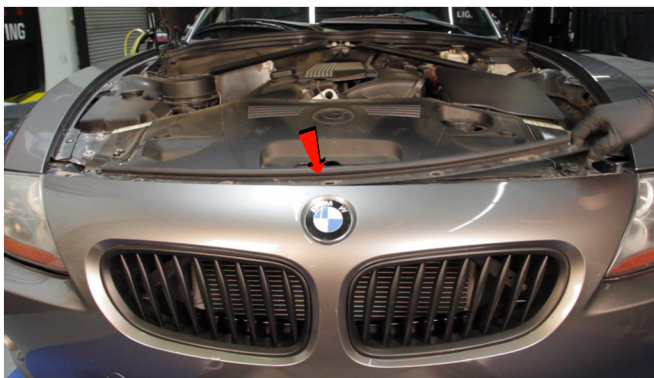
3) Remove the hood weatherstrip bracket.
