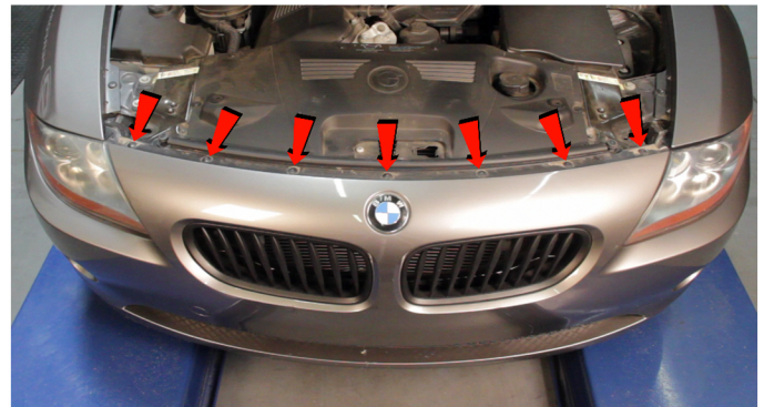
2) Remove [7x] T-30 Torx Bolts securing the fascia along the edge.
