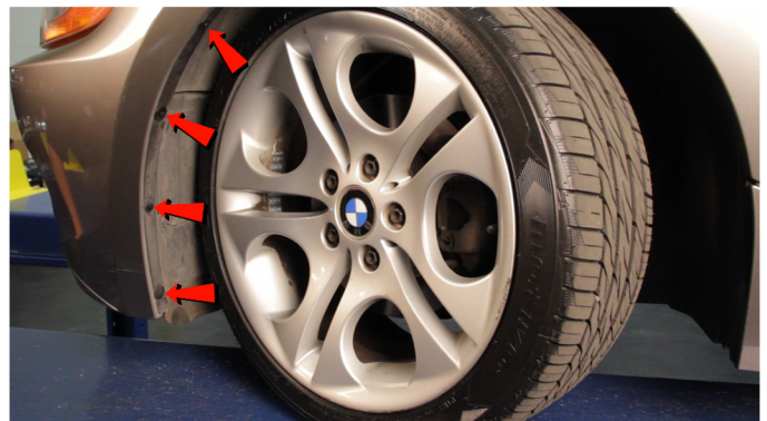
4) Remove the four plastic retainers securing the fascia at the wheel well using a panel popper.
