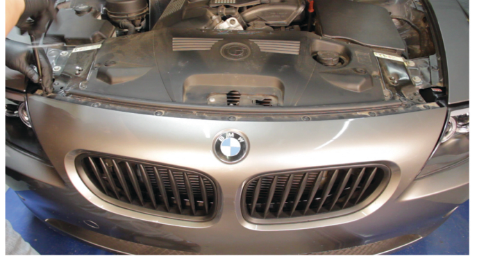
18) Reinstall [7x] T-30 Torx bolts to secure the hood weatherstrip bracket.
