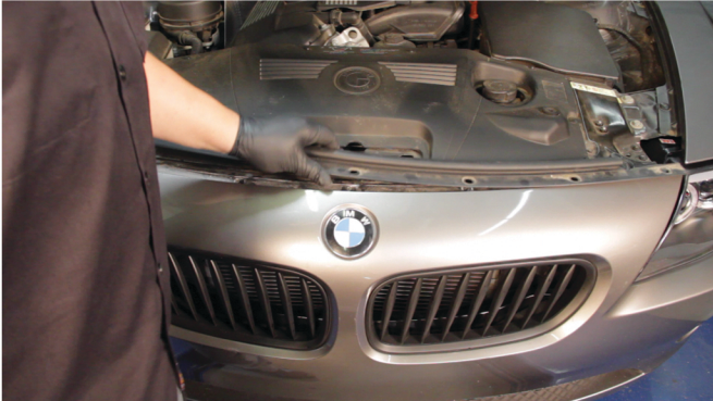
17) Replace the hood weatherstrip bracket.
